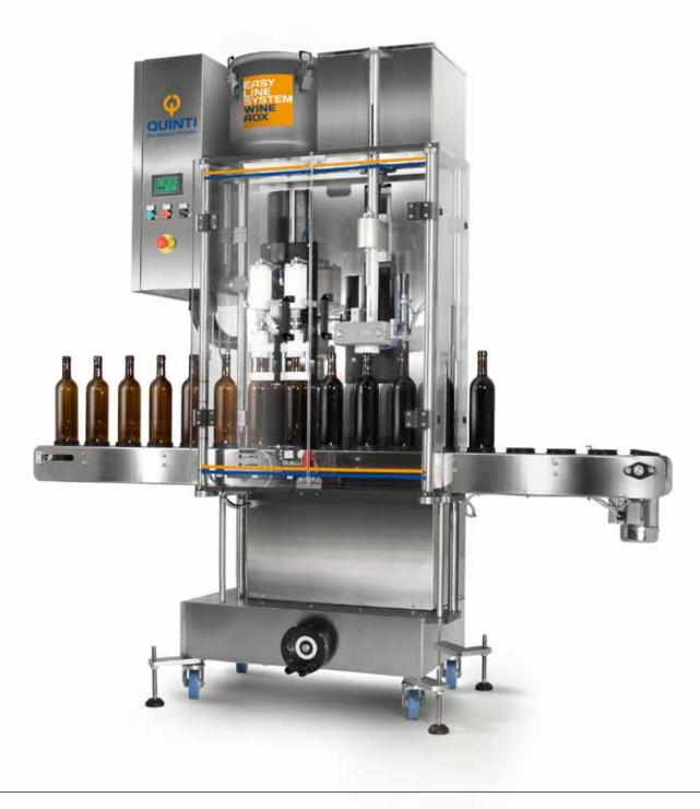
The **FILLING SYSTEM WITHOUT ISOBARIC OXYGEN-AOX** eliminates the air inside the bottle as much as possible. The AOX bottling machine can cap the bottles with a vacuum pump combined with an injection of nitrogen. One of the aim of the system is to limit the surplus and the dripping of beer and wine. This limits the formation of mould within the injector which is in turn decreases the amount of time and the cost of cleaning and maintaining of the machine.
